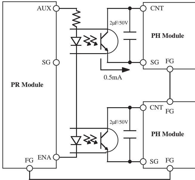
Figure 8-2 Recommended Circuitry for Parallel Operation of PR/PH Integration
