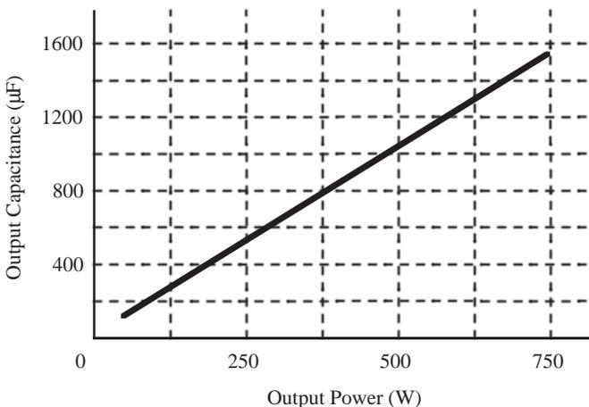
Figure 4-3 Minimum Capacitor Values vs. Output Power
