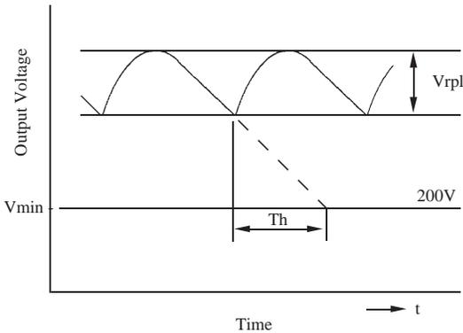
Figure 4-2 Ripple Voltage vs. Holdup Time
