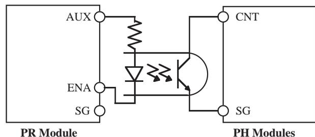
**Figure 8-1 Recommended Circuitry for PR/PH Integration**
