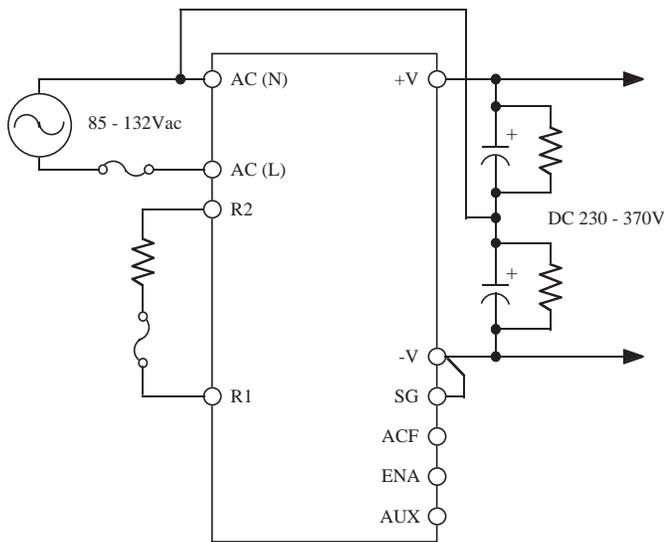
Figure 1-1 Voltage Doubler Connection
