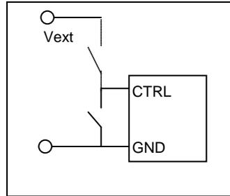
The product is equipped with a remote control function, i.e., the CTRL pin. The remote control can be connected to either the primary negative input connection (GND) or an external voltage (Vext). See Absolute Maximum Rating for maximum voltage level allowed at the CTRL pin.
