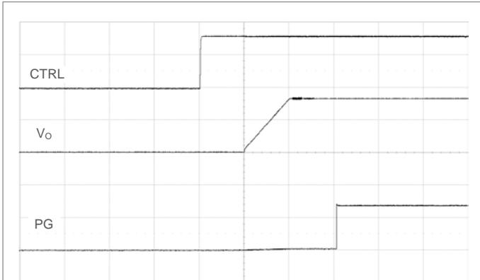
Start-up enabled by CTRL signal.  $\text{TON\_DELAY} = \text{TON\_RISE} = 10\text{ ms}$  (default).
