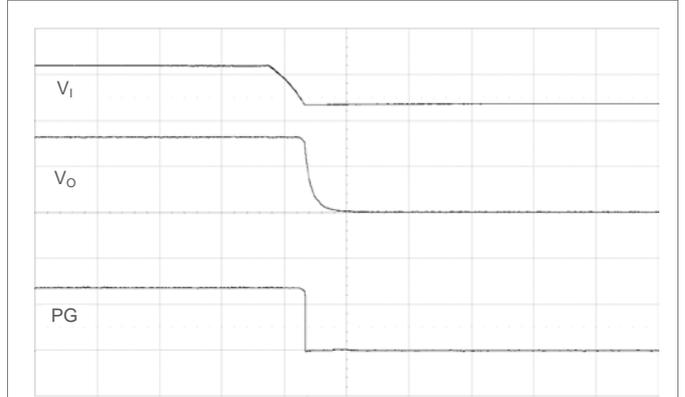
Shut-down by removing  $V_i$ .
