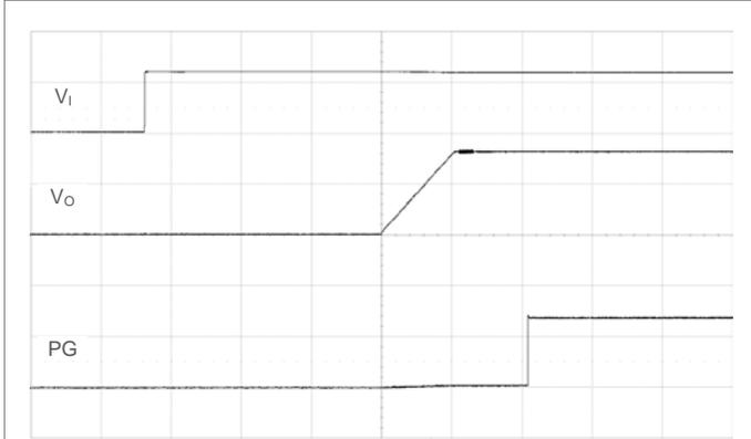
Start-up enabled by applying  $V_i$ .  $\text{TON\_DELAY} = \text{TON\_RISE} = 10\text{ ms}$  (default).
