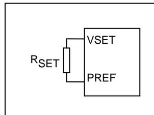
Using an external Pin-strap resistor, R<sub>SET</sub>, the output voltage can be set in the range 0.6 V to 5.0 V at 16 different levels shown in the table below. The resistor should be applied between the VSET pin and the PREF pin.
