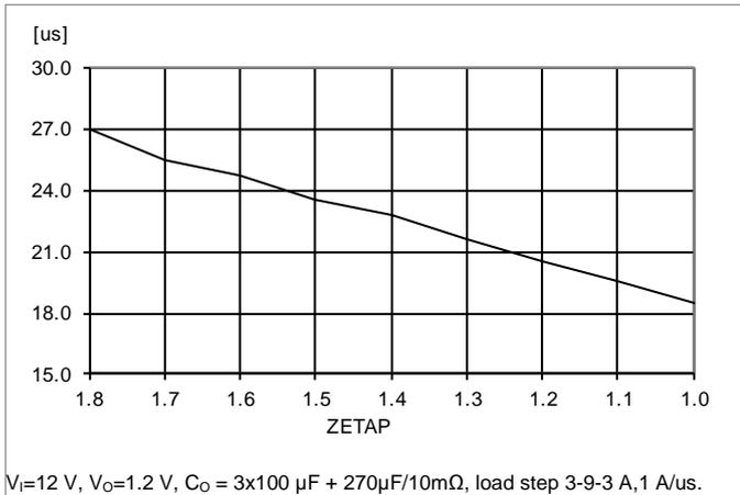
Recovery time to within 1% of V<sub>O</sub> vs. ZETAP setting.
